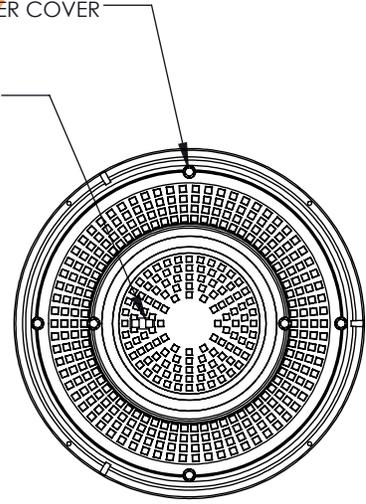
BOLT-DOWN ASSEMBLY WITH INNER COVER CLOSED PICK HOLE
